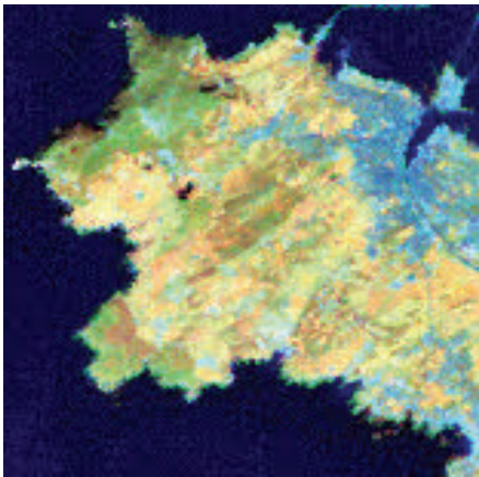
Landsat ETM+ : 25m spatial resolution 8 spectral bands Spectral range: 400-2100 nm
